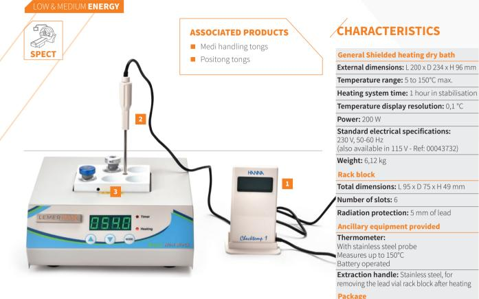
The shielded dry water bath is used during the heating stages of certain radiolabelling operations or reconstitution of cold kits with radioisotopes such as <sup>99m</sup>Tc. It can be installed on a benchtop, behind a screen, with its **5 mm lead shield**, or integrated into the Easypharma Compact<sup>®</sup> and 4R Low and Medium Energy hot cells or into the PSMEB. This high-precision digital dry block heater is microprocessor controlled with a setting resolution of one tenth of a degree.
