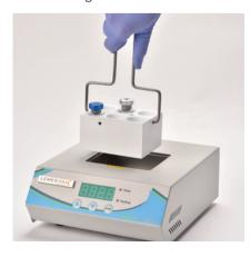
The set temperature, which can range from **5 to 150°C**, is automatically stored in the memory if the appliance is switched off or in the event of a power failure.
